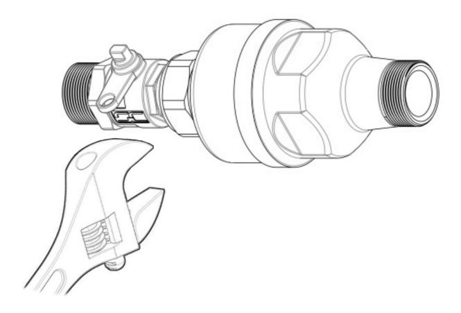
Flat faced meter unions are to be tightened between 9Nm and 15Nm which equates to a quarter to half a rotation with a spanner after being hand tightened.
